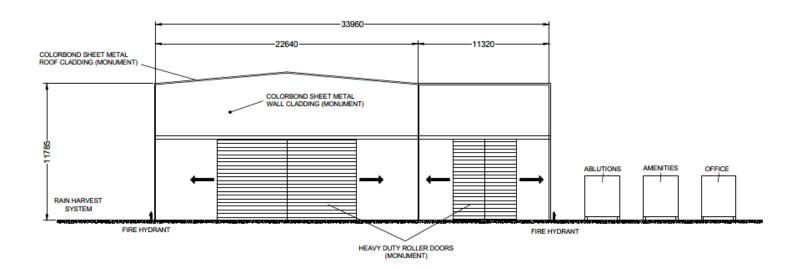
UAV EAST ELEVATION
